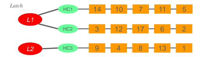
No. of hash buckets = init.ora parameter \_db\_block\_hash\_buckets No. of latches = \_db\_block\_hash\_latches
